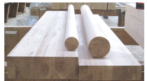
Beech glulam is another recent innovation PHOTO: SCHAFFITZEL + MIEBACH FASZINATION BRÜCKEN GMBH
